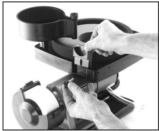
Figure 4. Mounting rest holder.
